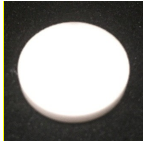
Figure 1: Synthetic micro-porous quartz glass. Left side 15mm diameter and 2mm thick sensor window.
