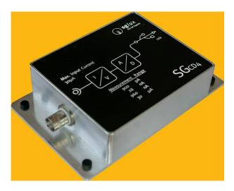
The SGCD4 is a switchable gain photocurrent digitizer that converts small DC currents (e.g. generated by photodiodes) into digital values transmitted via USB to a computer for displaying and recording. Four different current measurement ranges are user selectable by software. The device is delivered with a PTB traceable current calibration.
